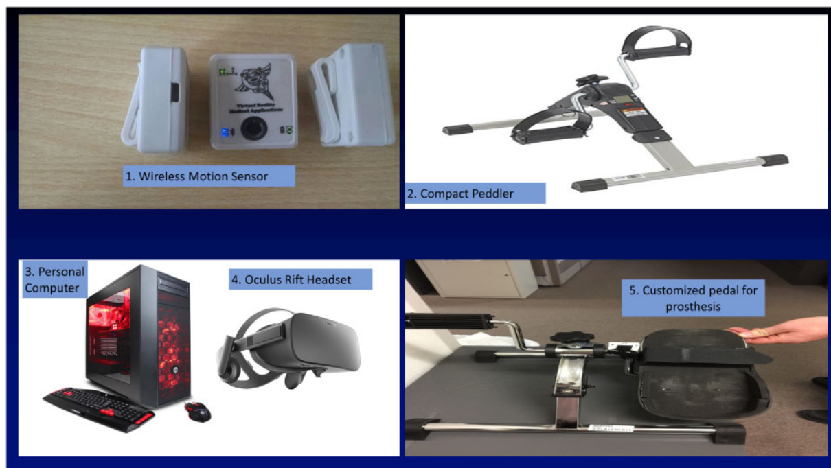
Figure 1. Illustration of the virtual reality treatment hardware, consisting of a motion sensor, bicycle pedaler, computer, Oculus headset, and prosthetic pedal.
